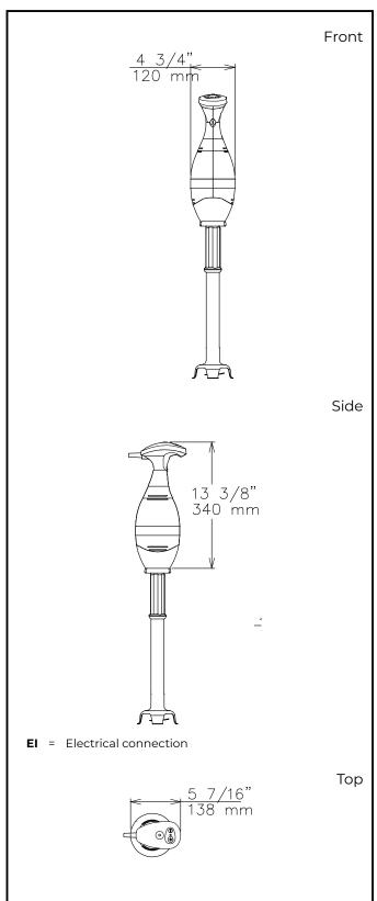
Electric Supply voltage: 602236 (DBP7555U) 110-120 V/1 ph/50/60 Hz **Total Watts:** 0.75 kW Plug type: USA NEMA 5-15P Key Information: External dimensions, Width: 5 7/16" (138 mm) External dimensions, Depth: 4 3/4" (120 mm) External dimensions, Height: 34 1/16" (865 mm) 11 7/16" (290 mm) **Shipping width:** Shipping depth: 27 3/16" (690 mm) **Shipping height:** 7 1/16" (180 mm) **Shipping weight:** 13 lbs (6 kg)
